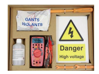
Fig. 2. An example of a set of equipment for a workshop servicing electric vehicles [50]
