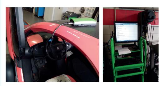
Fig 6. Bosch KTS connected to the vehicle
