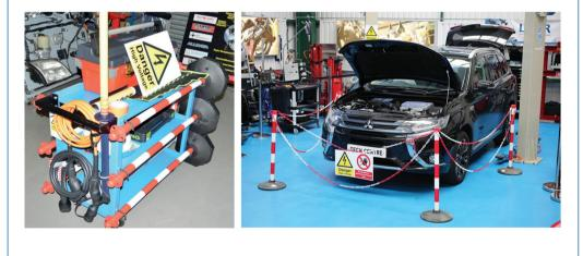
Fig. 3. Electric shock protection measures in the workshop [51]
